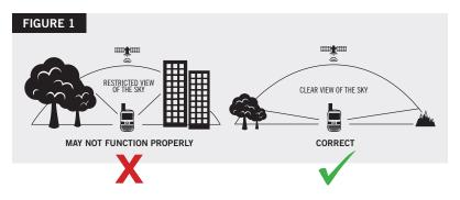
Orienting SPOT X vertically with the antenna facing towards the sky, will improve performance as the antenna is located on the top portion of the device.
