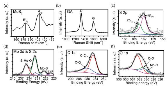
Figure 3. a,b) Raman spectra of the hybrid aerogel. X-ray photoelectron spectra of the MoS<sub>2</sub>/graphene hybrid aerogel: c) S 2p; d) Mo 3d and S 2s; e) C 1s; f) O 1s.
