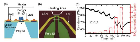
Figure 4. a) Cross-sectional schematic of the microheater sensor. b) Optical image of one microheater showing the Pt/Ti sensing electrodes above the polysilicon heater. c) Real time response of the sensor at room temperature toward different  $NO_2$  concentrations.
