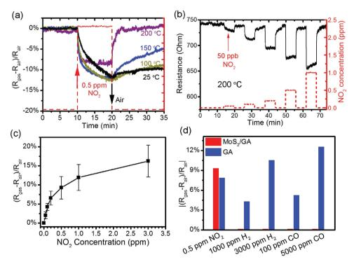
Figure 5. a) Sensor response to 0.5 ppm  $NO_2$  at various microheater temperatures, displaying improvement in response and recovery time. b) Real-time resistance change of the sensor with the microheater temperature of 200 °C. c) Response versus  $NO_2$  concentration for microheater temperature of 200 °C. d) Selectivity of the  $MoS_2/GA$  sensor compared to GA alone for microheater temperature of 200 °C.
