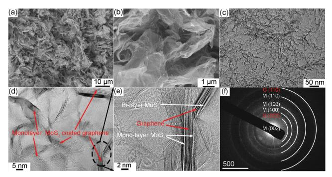
Figure 2. Morphology of the as-prepared  $MoS_2/GA$ . a,b) SEM images of the hybrid aerogel with different magnifications. c) Low magnification TEM image of the  $MoS_2/GA$ . d) High resolution TEM image of the  $MoS_2/GA$ , showing most of the graphene is coated by monolayer  $MoS_2$ . e) Enlarged TEM image demonstrating the  $MoS_2$  coating of the few-layer graphene scaffold. f) Relevant selected area electron diffraction (SAED) pattern of the  $MoS_2/GA$ .
