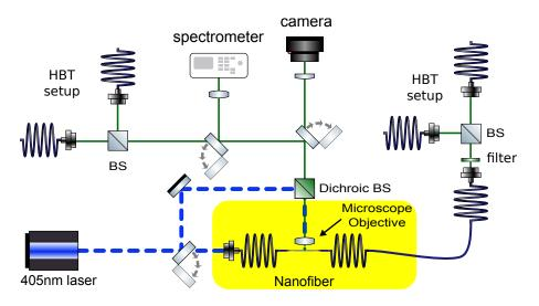
Figure 3.14: Setup for the nanofiber experiment: a blue pulsed laser can excite the emitter both from the nanofiber and from freespace. The image and the spectra of the nanocrystals can be recorded using a camera. Ultimately, it is possible to perform the  $g^{(2)}$  measurement in both configurations. The part surrounded by in yellow is placed in a box under a clean laminar air-flow. BS: non polarizing beamsplitter, HBT: Hanbury Brown and Twiss.
