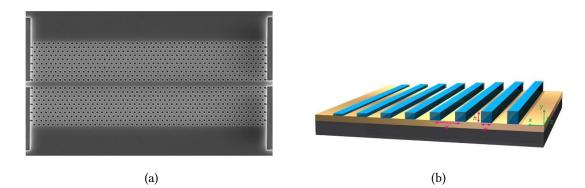
Figure 1.14: Sanning electron microscopy image of a photonic crystal waveguide array 1.14a (*credits: García-Rupérez* et al. [59]) and scheme of an array of surface plasmon polariton waveguides (PMMA on gold surface) 1.14b (*credits: Block* et al. [60]).
