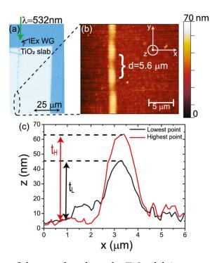
Figure 4.11: (a) Image of the sample, where the  $TiO_2$  slab is present, (b) obtained atomic force microscope image, showing a modulation of the thickness of the resin with a periodicity of 5.6 µm; (c) profile of the fabricated ridge; the red one is taken where the thickness of the ridge is maximal, while the dark one was taken were the thickness of the ridge is minimal. (*credits: Lio* et al. [115]).
