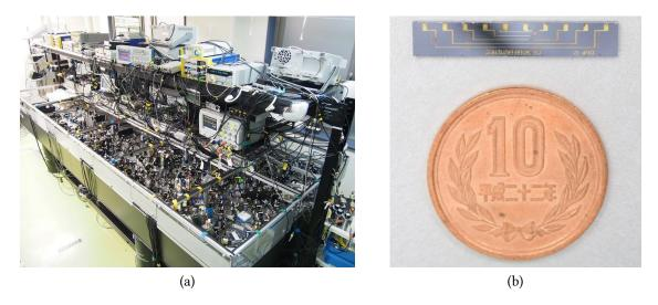
Figure 1.13: Difference between freespace (a) and integrated (b) optics. The free-space optics is flexible and historically well known, but requires fine alignment and wide space. On the contrary, integrated optics cannot be modified one fabricated, but it is small, stable and does not risk misalignment.
