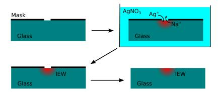
Figure 4.7: Fabrication procedure of Ion-exchange glass waveguide: first of all, a mask is created on the surface of a glass plate; then the glass is immersed in a solution containing  $Ag^+$  ions, as for example a solution of  $AgNO_3$ . Some of the  $Ag^+$  ions replace some of the  $Na^+$  of the glass, modifying its refraction index. Eventually the support is extracted and the mask is removed.
