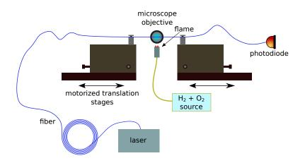
Figure 3.10: Experimental setup for pulling nanofibers. The laser is used to constantly monitor the transmission during the process.
