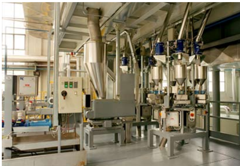
The "gravimetric feeders" feed in the ingredients.
