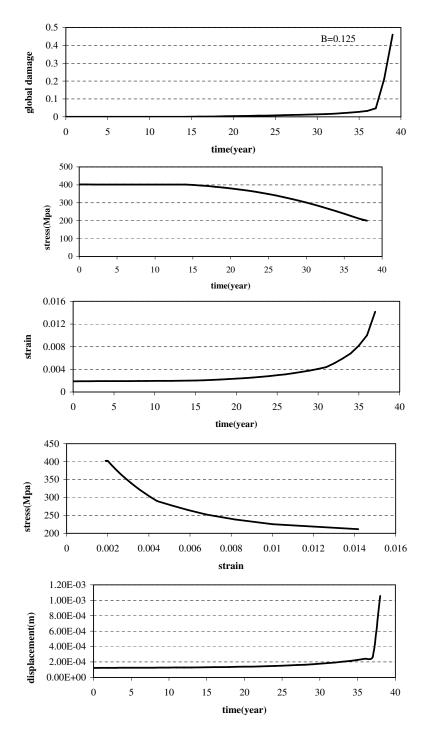
Figure 5. Global damage, displacement of node 1, and major principal stress, major principal strain, and stress-strain relationship of element 99, respectively, of the notched bar (B = 0.125).
