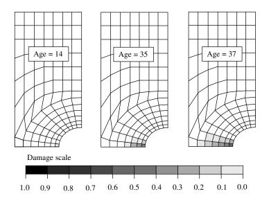
Figure 9. Damage patterns of the plate (B = 0.125).
