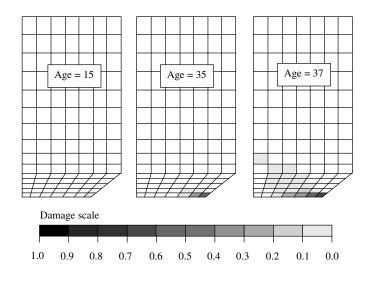
Figure 4. Damage patterns of the notched bar (B = 0.125).
