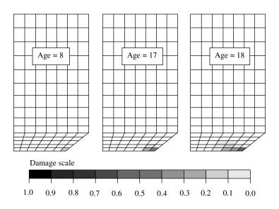
Figure 6. Damage patterns of the notched bar (B = 0.25).
