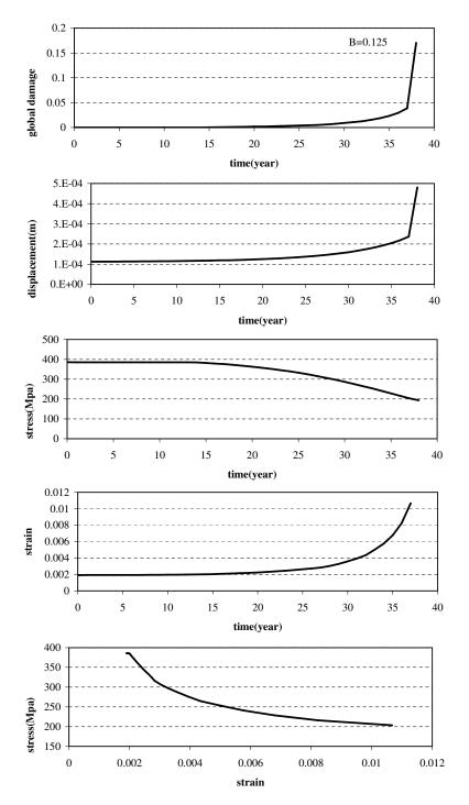
Figure 10. Global damage, displacement of node 1, and major principal stress, major principal strain, and stress-strain relationship of element 92, respectively, of the notched bar (B = 0.125).
