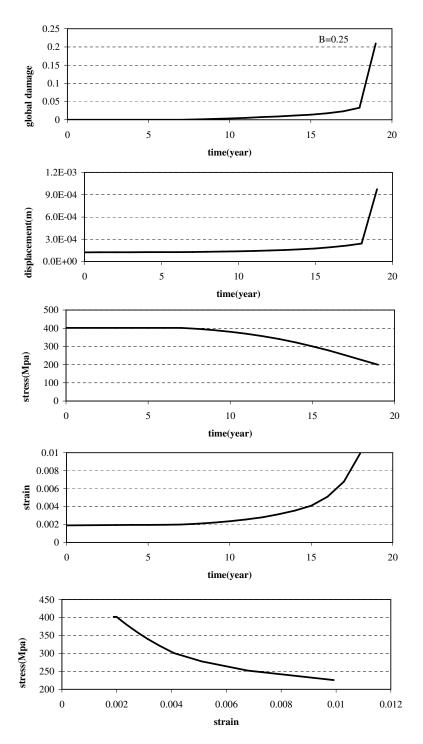
Figure 7. Global damage, displacement of node 1, and major principal stress, major principal strain, and stress-strain relationship of element 99, respectively, of the notched bar (B = 0.25).
