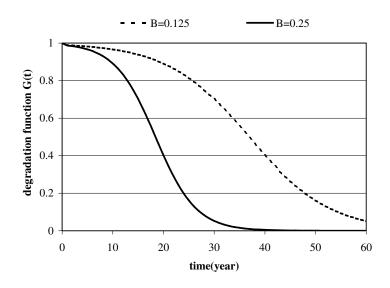
Figure 3. Degradation function of steel.
