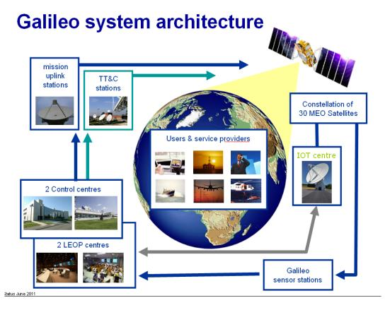
Galileo also depends on an extensive ground infrastructure, which will have to make sure that time and positioning data are extremely accurate — a single billionth of a second clock error means a positioning error up to a range of 30 cm. This ground
