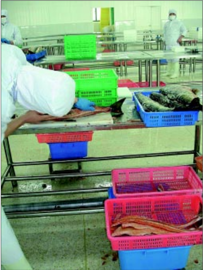
Station 1. Filleting dressed (headed and gutted) salmon. Fish are cut in half lengthwise and the vertebrae removed.
