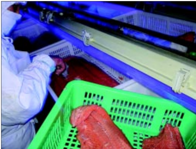
Station 4. Parasite removal under ultraviolet (UV) light. About 20 people were working with tweezers to remove parasites visible from the surface, mostly in the belly area. UV light is necessary to spot parasites when working with salmon. Chum are said to have a particularly high number of parasites.
