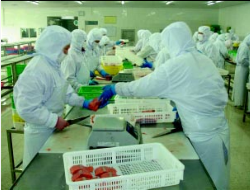
Station 5. Cutting into individual portions for freezing. Fillets are cut and weighed according to client specifications. They are then placed on trays for freezing in a plate freezer.
