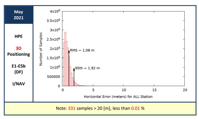
Figure 20: Horizontal Positioning Error (HPE) for "Galileo-only" users in May 2021
