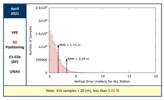
Figure 22: Vertical Positioning Error (VPE) for "Galileo-only" users in April 2021
