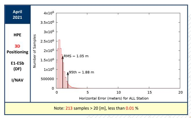
Figure 19: Horizontal Positioning Error (HPE) for "Galileo-only" users in April 2021
