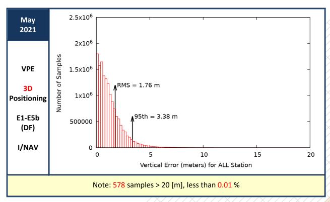
Figure 23: Vertical Positioning Error (VPE) for "Galileo-only" users in May 2021
