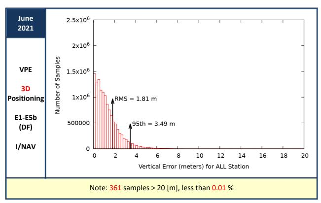
Figure 24: Vertical Positioning Error (VPE) for "Galileo-only" users in June 2021
