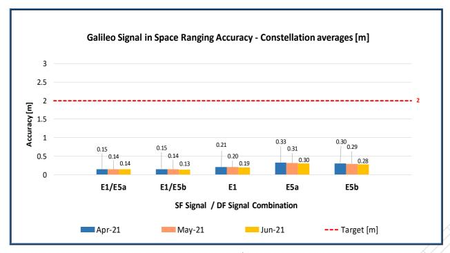
Figure 8 : Monthly Galileo SIS Ranging Accuracy (95<sup>th</sup> percentile) "over all satellites" (constellation average), measured during the reporting period
