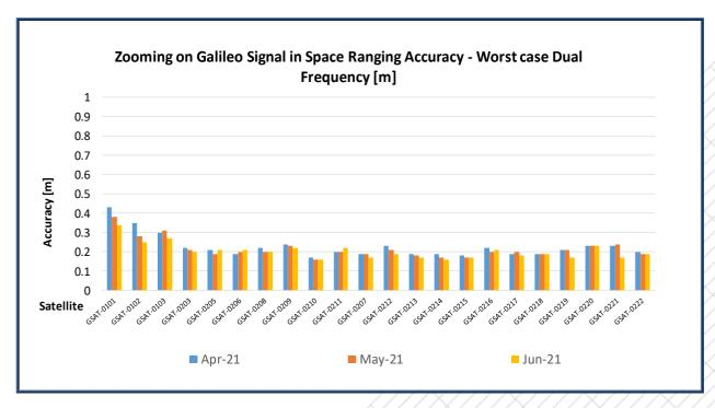
Figure 6 : Monthly Galileo SIS Ranging Accuracy (95<sup>th</sup> percentile) "for any satellite", measured during reporting period for worst-case, Dual-Frequency (DF)
