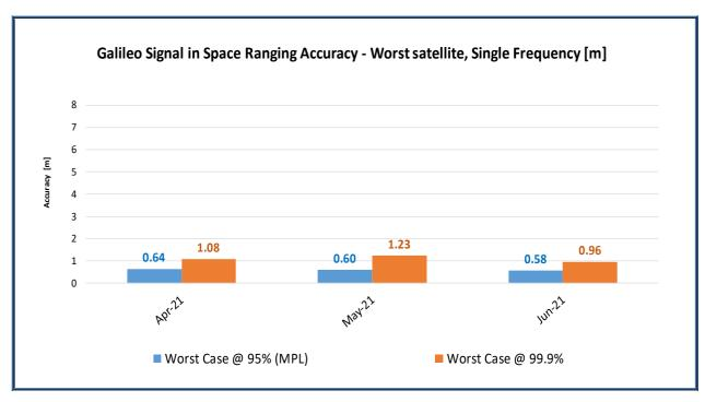
Figure 5 : Worst-case, monthly Galileo SIS Ranging Accuracy (at 95<sup>th</sup> and 99.9<sup>th</sup> confidence level percentiles) "for any satellite", any SIS (SF and DF combinations)
