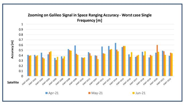
Figure 7 : Monthly Galileo SIS Ranging Accuracy (95<sup>th</sup> percentile) "for any satellite", measured during the reporting period for worst-case, Single-Frequency (SF)
