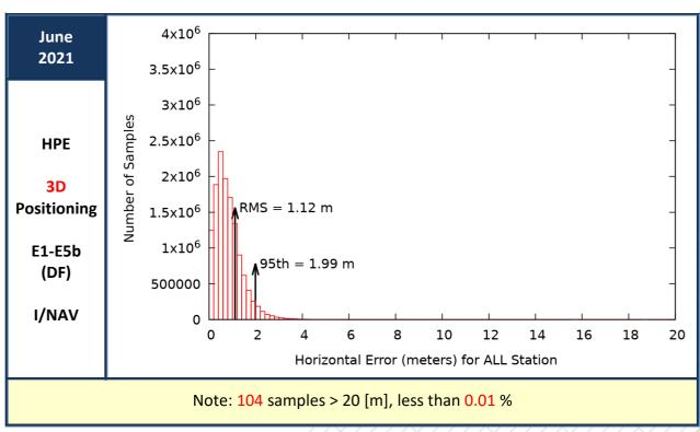
Figure 21: Horizontal Positioning Error (HPE) for "Galileo-only" users in June 2021
