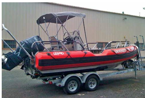
Figure 4.31. Example of a Rigid-Hull Inflatable Boat. The USAP version would likely have an enclosed wheelhouse, given the prevailing temperature and weather conditions in the vicinity of Palmer Station. Source: Tim McGovern.
