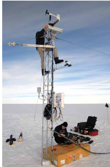
Figure 4.7. Weather instruments and Global Positioning Systems being placed on uncrevassed ice next to the Pine Island Glacier to allow near continuous observations of the weather conditions and to monitor its movement. This is an example of the programs considered during the NSF-sponsored workshop on “Autonomous Polar Observing Systems” (2010). Source: Cliff Leight.
