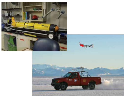
Figure 4.2. (top) Underwater glider used for autonomous ocean research. Source: Don Hartill. (bottom) Modern aerial drone for wide-area observations. Source: John Cassano.
