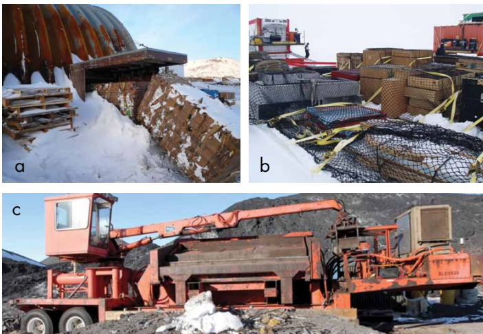
Figure 4.50. (a) Consolidated waste, in this case baling cardboard waste, at McMurdo Station for shipment off continent. (b) South Pole waste materials are returned to McMurdo Station, in the case shown via the return trip of the traverse. (c) Processing metal waste at McMurdo Station. Sources: (a) Lisa Harding; (b) Paul Thur; (c) USAP photo archives.
