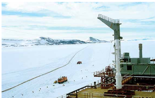
Figure 16. When ice conditions in McMurdo Sound made the approach to the pier so difficult that the tanker could not make it to the pier, the fuel was off-loaded over the sea ice via hoses. The USAP recognized this vulnerability and has since decreased fuel usage and increased fuel storage capacity so that it now has a two-year supply on hand.
