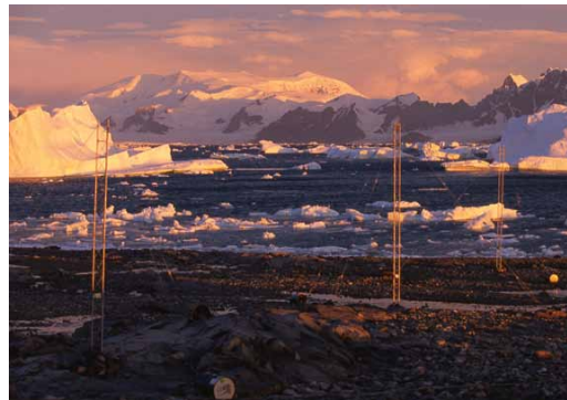
Figure 4.71. The U.S. HF meteor radar array at the U.K.'s Rothera research station, used to study thermospheric winds. Source: David Fritts.
