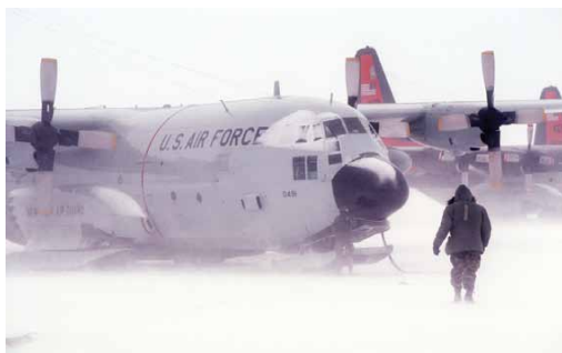
Figure 4.42. Air National Guard crew maintaining an LC-130 at the McMurdo airstrip, air temperature -7^{\circ}\text{F} ( 22^{\circ}\text{C} ), winds 17 miles per hour (15 knots). Source: USAF Air National Guard.
