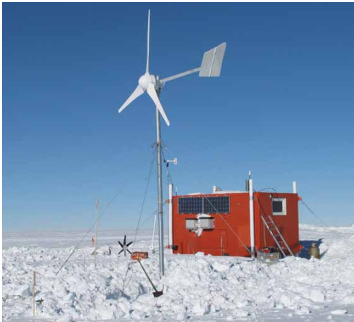
Figure 3.13. Photo of an Automatic Geophysical Observatory from the rear, with two solar panels and close-up of the wind generator. These stations operate year-around, unattended, under sun and wind power. Source: Siena College and New Jersey Institute of Technology.
