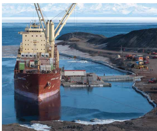
Figure 4.24. Unloading cargo in February 2012 from the Military Sealift Command cargo ship Green Wave via the portable modular causeway system supplied and operated by the U.S. Army 331 st Transportation Company. Source: William Henriksen.
