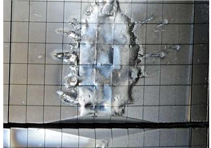
JET runaway electrons damage. https://www.iter.org/newsline/-/2234
