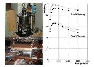
Fig. 4 – On the left we see photographs of the GSI TAS and *Lucrecia*. On the right we see the corresponding total and photopeak efficiency curves for these two detectors. The empty and filled points represent the results for the GSI TAS and *Lucrecia* respectively.
