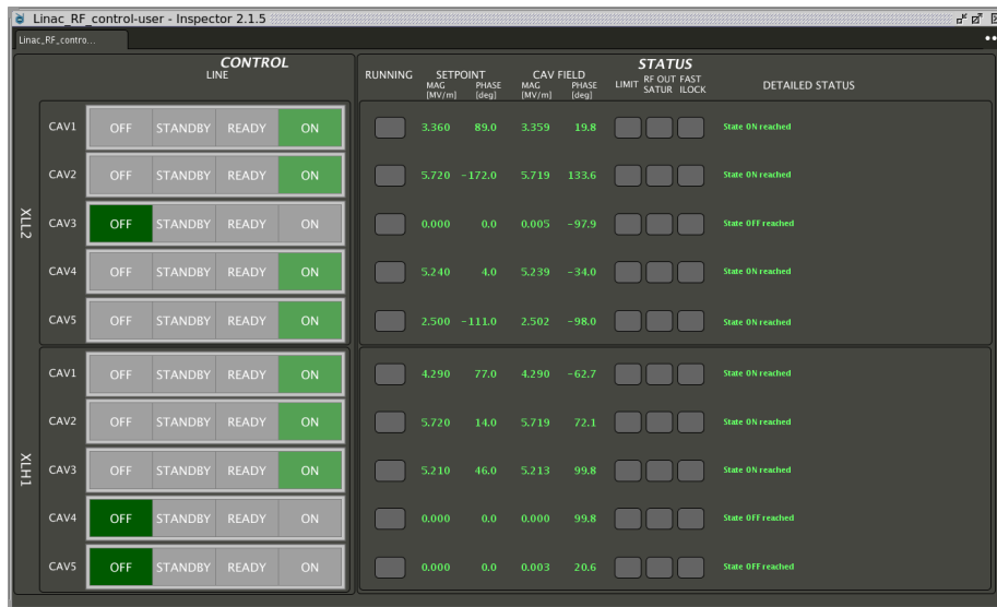
Figure 36: The control panel for the cryomodules. Here XLL2.CAV3, XLH1.CAV4 and XLH1.CAV5 are switched off.
