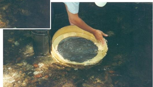
Figure 3.4.19. Washing thoroughly with water all the stream sediment sampling equipment. Photographs: Alecos Demetriades (IGME/IUGS-CGGB).
