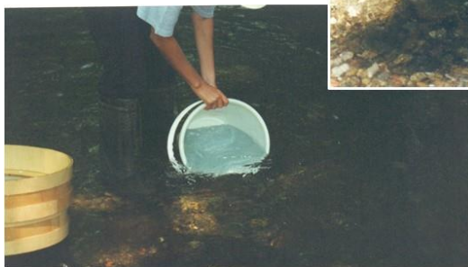
Figure 3.4.19. Washing thoroughly with water all the stream sediment sampling equipment. Photographs: Alecos Demetriades (IGME/IUGS-CGGB).
