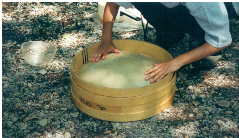
Figure 3.4.5. Setting up the circular collection pan, the 0.150 and 2 mm sieve on a stable position; the collection pan is below the bottom sieve 4 . Photograph: Alecos Demetriades (IGME/IUGS-CGGB).
