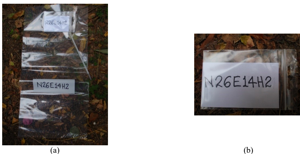
Figure 3.2.15. Photographs showing numbered (a) Certified trace-element free plastic Rilsan® bag with a plastic strip lock for packing the humus sample (Step (i) of humus sampling procedure – see Section §3.2.4.3), and (b) Small card in a plastic zip-lock bag (Step (ii) of the sampling procedure for Humus, see Section §3.2.4.3). Photographs: Alecos Demetriades (IGME/IUGS-CGGB).
