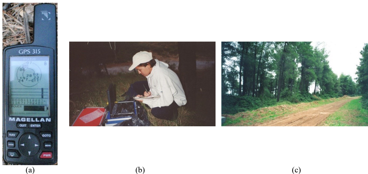
Figure 3.2.8. Photographs showing (a) GPS instrument and (b) Laptop with GPS for recording sample site coordinates – Step (i) of sampling procedure (see Section §3.2.4.2). The reason for switching on the GPS upon reaching the sample site is that in a few remote and forested areas it takes some time to locate the satellites. If the GPS is struggling to find the three satellites to triangulate the sample site coordinates without success, as in this case, move it a few metres to an open space or the nearest forest track road (c). Photographs: Alecos Demetriades (IGME/IUGS-CGGB).
