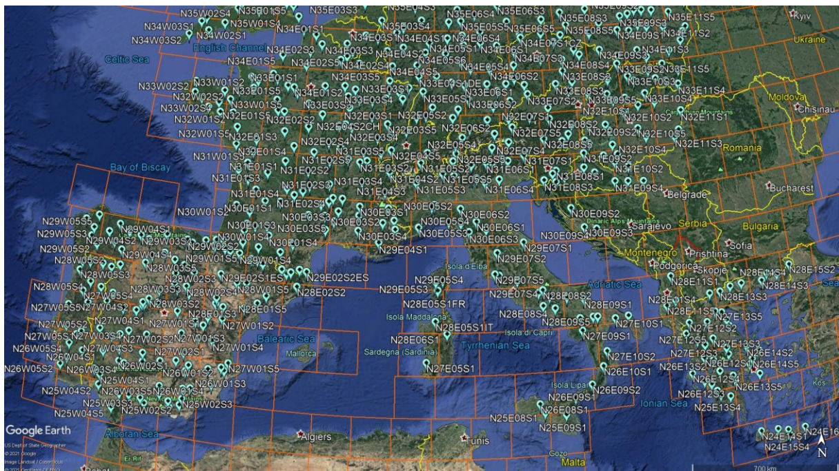
Figure 9.12. Google Earth image showing the stream sediment sample sites with their identification numbers, FOREGS Geochemical Atlas of Europe (Salminen et al., 2005). The orange squares are the 160x160 km GTN grid cells. Plotted by Alecos Demetriades (IGME/IUGS-CGGB) with Golden Software's MapViewer™ v8 and exported to a kml format file for display on Google Earth.
