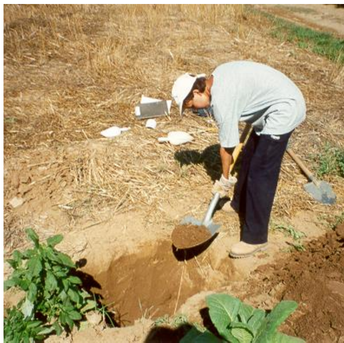
Figure 3.5.10. Digging a pit on the floodplain for the collection of the floodplain sediment sample, NW Peloponnese, Hellas. It is noted that this is not a suitable site for the collection of the top floodplain sediment sample because it is cultivated. In this case, only the bottom sample was collected from the pit, and the top sample from a nearby undisturbed site. Photograph: Alecos Demetriades (IGME/IUGS-CGGB), FOREGS Geochemical Atlas of Europe (Salminen et al., 2005).
