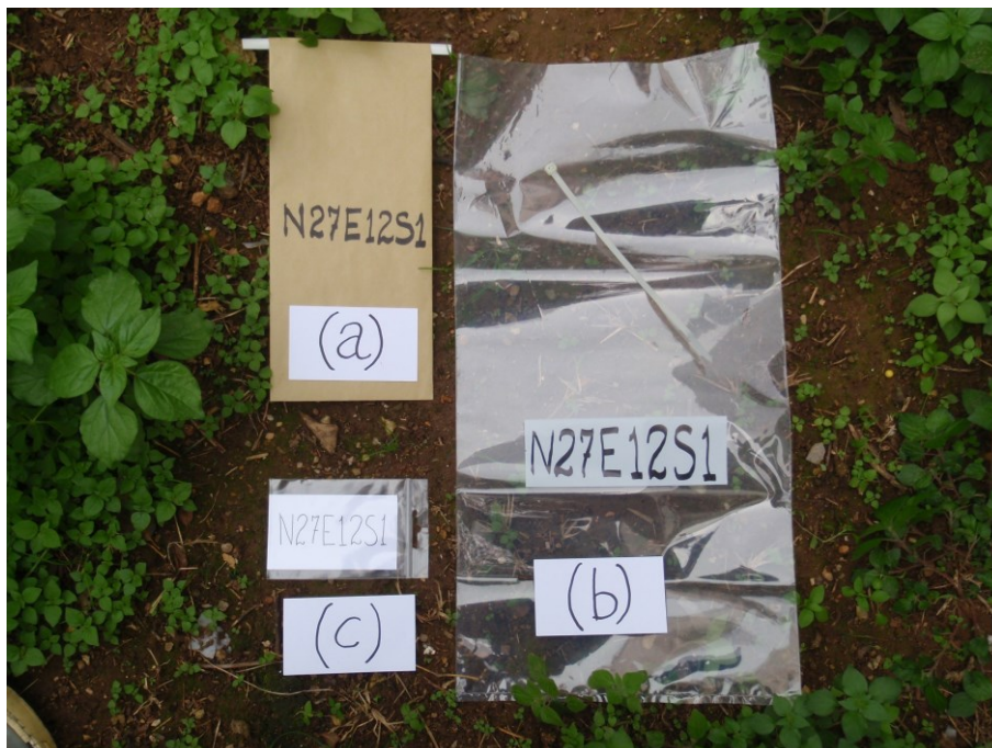
Figure 3.4.2. Write stream sediment sample number with a black permanent ink marker on either (a) Wet strength Kraft paper bag (12.5x25 cm) with a plastic-coated aluminium tin tie for sealing bag, or (b) Strong certified trace-element free plastic bag (300x600 mm) that is secured with a plastic strip lock, and (c) Write sample number on both sides of a small card (6x10 cm), and place card in a small plastic zip-lock bag (7.5x11.5 cm) and seal it. Photograph: Alecos Demetriades (IGME/IUGS-CGGB).
