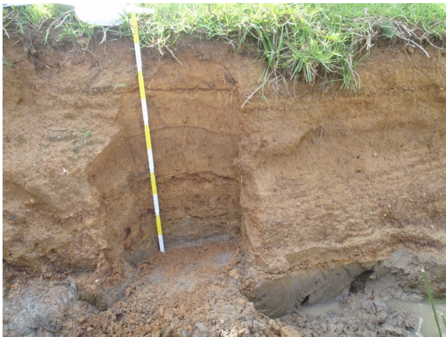
Figure 3.5.15. Overbank sediment section, S33E180, Cape Farms (18.610533°E, 33.684647°S), Cape Town, South Africa, field-training course on the occasion of the 35 th International Geological Congress in Cape Town; the bottom sample is collected from the 15-cm thick overbank sediment layer above the grey layer (reducing conditions - gleying), which is below the stagnant water level, and the top sample is taken from the surface layer after removing the grass. Photograph: Alecos Demetriades (IGME/IUGS-CGGB).
