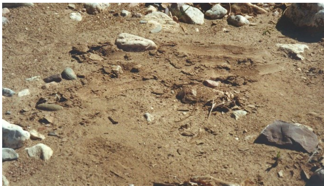
Figure 3.4.21. Moist stream sediment, N25E13W2S (22.43°E, 37.09°N), FOREGS Geochemical Atlas of Europe, Hellas. As it is not possible to sieve in-situ the stream sediment, enough moist stream sediment should be collected to yield at least 1000 grams of <0.150 mm dry stream sediment. Photograph: Alecos Demetriades (IGME/IUGS-CGGB).
