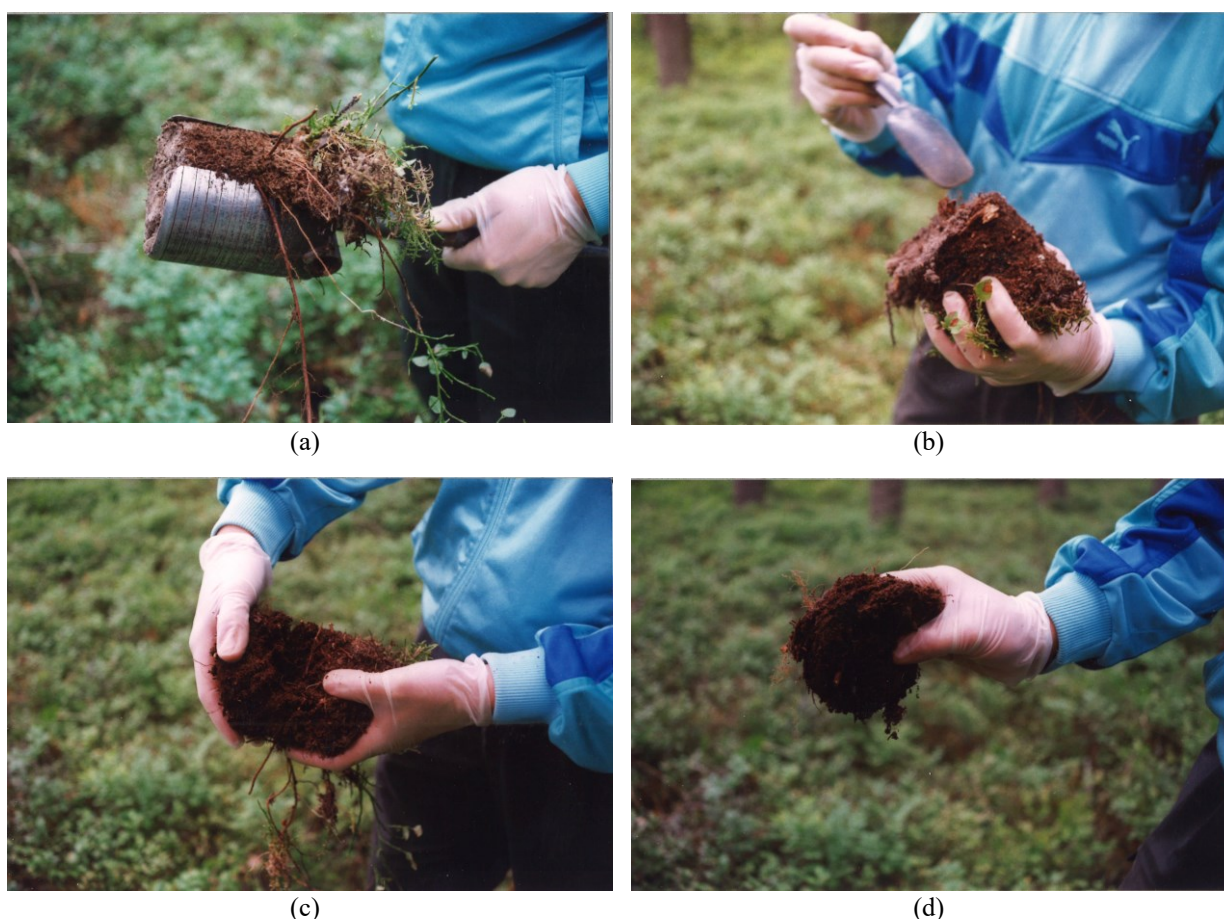
Figure 3.2.16. (a) Humus sampling in Finland using cylindrical sampler. (b) Removal of all mineral soil with a plastic scoop. (c) Pull apart Humus (on left) and roots (on right), and (d) Final Humus sample for bagging in either certified trace element free Rilsan® bag or white cotton bag free of chemical impregnation; when full the small-numbered card in a plastic zip-lock bag is placed on top, and the plastic bag is secured with the plastic strip lock or the cotton bag is securely tied with the drawstring. Photographs: Timo Tarvainen, Geological Survey of Finland (Salminen, Tarvainen et al., 1998, Figs. 8a to 8d, p.23-24).
