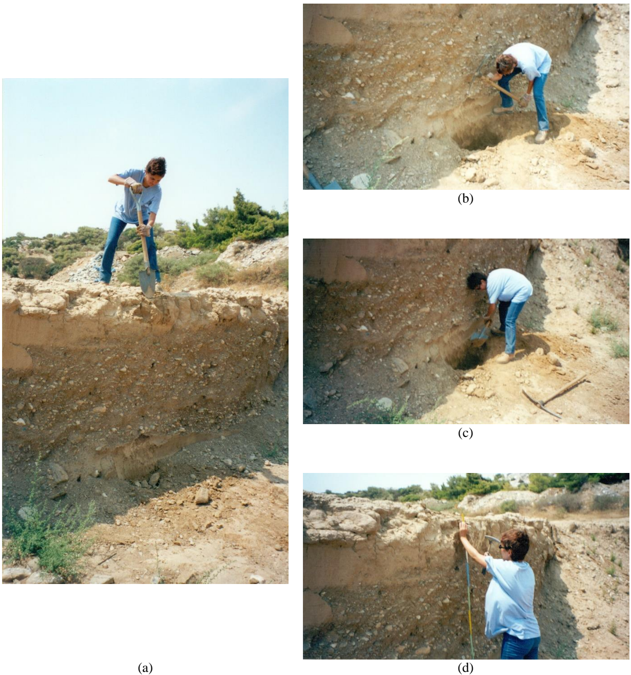
Figure 3.5.18. (a) Cutting a vertical profile in the exposed section of the overbank/floodplain sediment sequence; note the alternate layers of fine-grained overbank sediment and sand with gravel, denoting low and high energy environments, respectively. (b) and (c) Digging a pit at the base of the exposed section to locate other lower fine-grained overbank sediment layers. (d) Placing the wooden measure on the face of the overbank sediment sequence. It is noted that due to the prevailing dry conditions in the eastern Attiki region, this particular river has not flooded for many years, and is continuously downcutting its valley to reach the base level, thus exposing the overbank/floodplain sediment sequence. Photographs: Alecos Demetriades (IGME/IUGS-CGGB), FOREGS Geochemical Atlas of Europe project, Lavreotiki peninsula, Attiki (N26E14F6; 24.055°E, 37.755°N), Hellas (Salminen et al., 2005).
