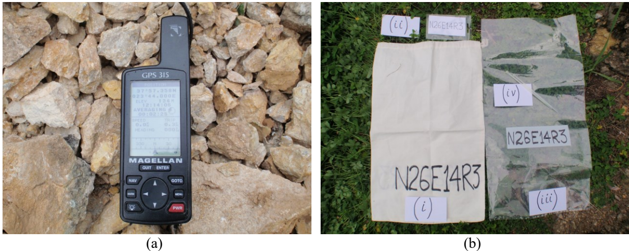
Figure 3.1.6. (a) Switch on the GPS unit to record the sample site coordinates (23.733333°E, 37.955967°N). (b) Bags and other equipment for the collection of rock sample N26E14R3, Aghios Ioannis Hill, Athens, Hellenic Republic: (i) Sample number written with a black permanent ink marker on a 27x45 cm cotton bag with drawstring; (ii) Sample number written with a black permanent ink marker on both sides of a 6x10 cm white card and placed in a 7.5x11.5 cm plastic zip-lock bag; (iii) Sample number written with a black permanent ink marker on a strong certified trace element free 25x50 cm Rilsan ® bag (used instead of the cotton bag), and (iv) Two plastic strip locks for securing bags.
