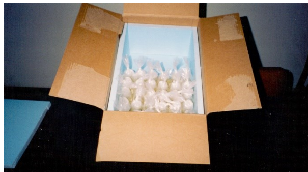
Figure 3.3.7. Samples of stream water are packed in a strong carton box with insulating material boards (blue) in order to retain a low temperature during the transportation of the samples to the laboratory. Note: Addition of dry ice or ice cubes may be necessary, especially under hot environmental conditions. Photograph: Alecos Demetriades (IGME/IUGS-CGGB).
